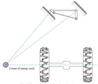
Fig.5. Steering Mechanism Design.
