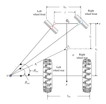
Fig.6. Geometry left wheel front angle by Ackermann steering theory.
