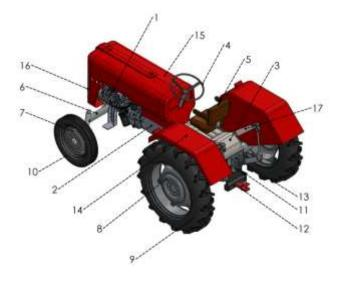
Fig.4. The main driveline units of the medium-sized-purpose vehicle.
